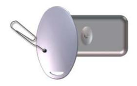
**9-**THE "AIR4" LED WILL FLASH RAPIDLY; PRESS THE BUTTON BY WHICH THE CODE WILL BE MEMORISED AND HOLD DOWN UNTIL THE LED GOES OUT.
