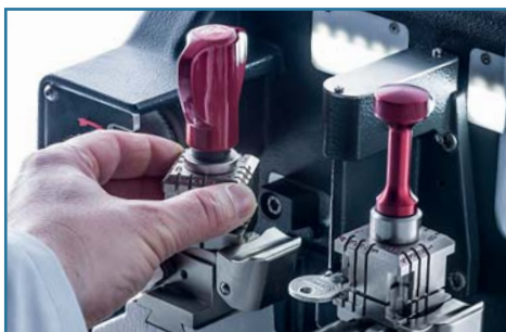
Four-sided, nickel plated clamps
