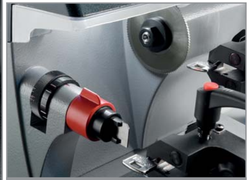
HSS cutter able to reach a speed of 650 rpm
