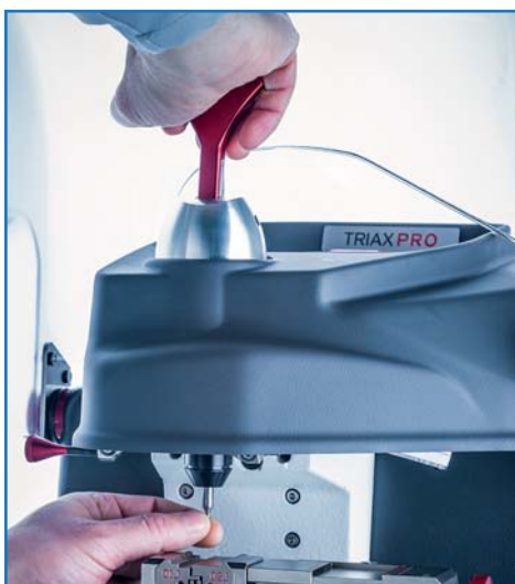
Optimized cutter change system
